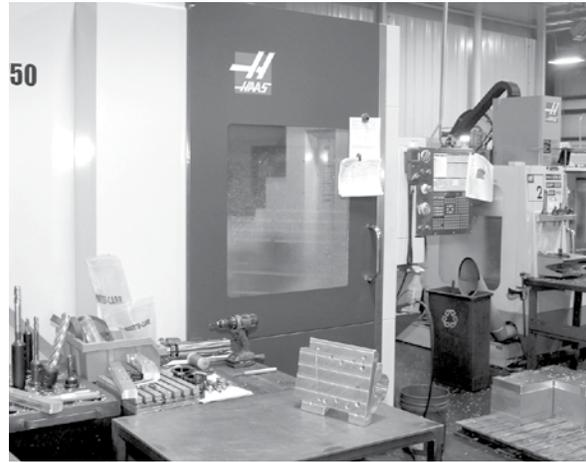
Left: A Haas UMC-750 5-axis machining center at Creative Blow Mold Tooling.
