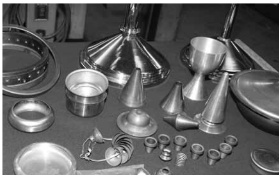
Above: Examples of spun parts produced at United Metal Spinning in KCMO.
