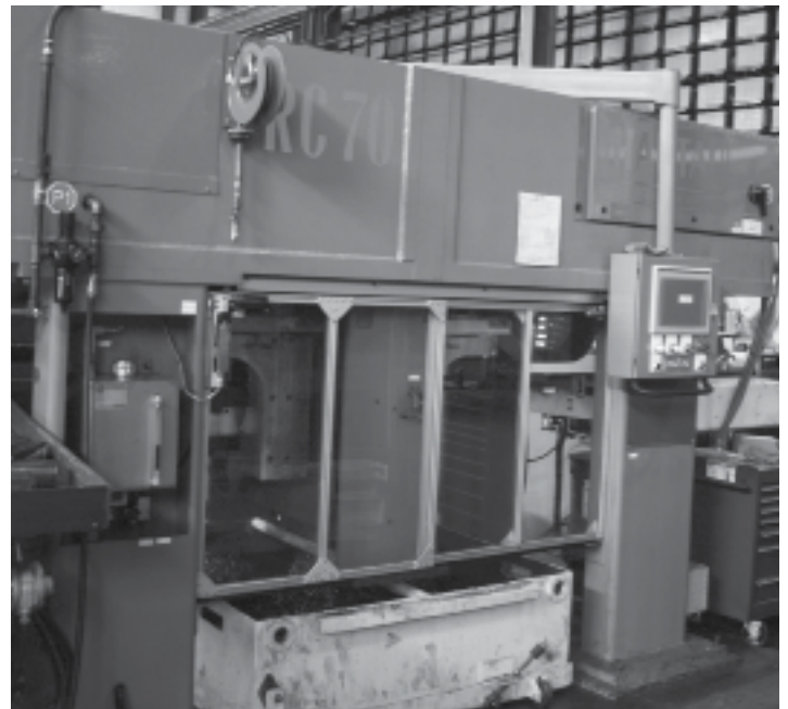
Above: The new Hautau RC70 CNC tube cutting system at EMJ-KC. It can cut tube up to 7" in diameter with 7/8" walls.
